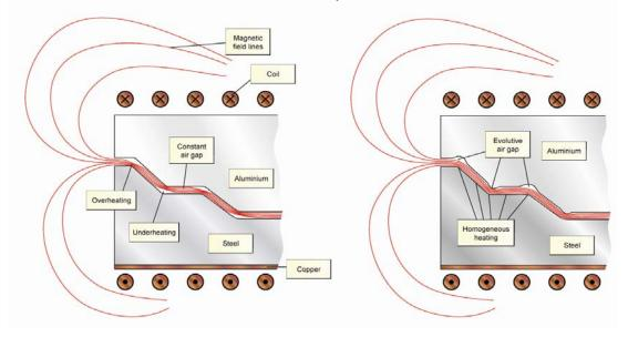
Fig. 5 Effect of air-gap on the magnetic field. Therefore, to detail the relationship (8), in generating variable air-gaps, at our convenience we
